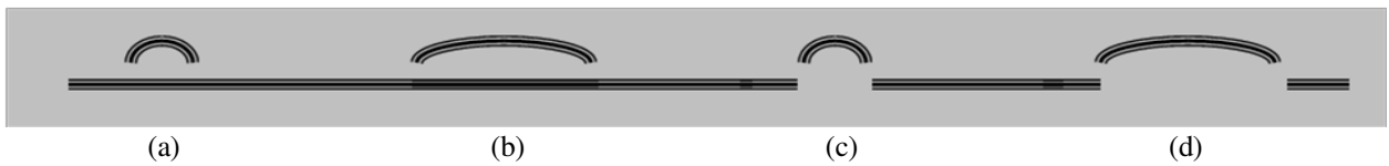
Figure 7. Schematic representation of four different characteristic Multi-Skip wall loss responses resulting from four different wall loss areas (time axis vertical and scan direction horizontal).
