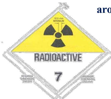
Placard for vehicles and should post around all 3 direction of the vehicle
