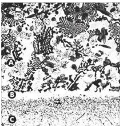
Metallurgical bonding with no dilution A: Deposit , B: Diffusion zone, C: Base metal
