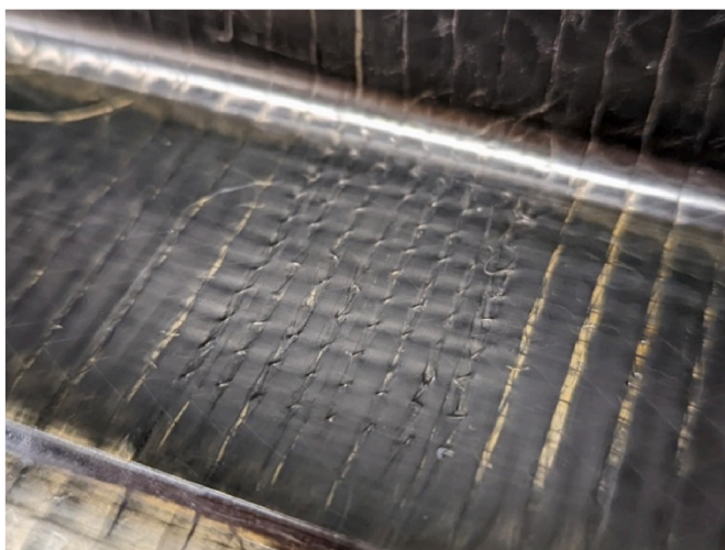
Fig. 2. Illustration of 3.44 mm spaced tufting on the carbon-epoxy composite T-joint.
