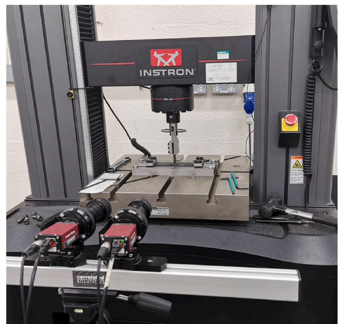
Fig. 4. DIC setup and mechanical testing configuration.
