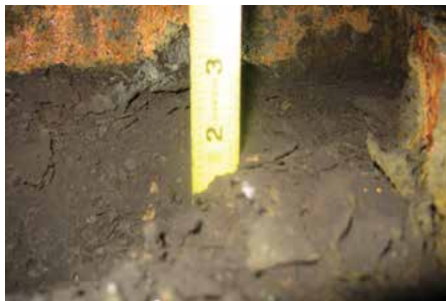
▲ Figure 6. Deposits accumulate on tray decks, especially under downcomers and in seal and draw pans. These deposits accumulate during process operations and/or are flushed from other surfaces during shutdown washes.
