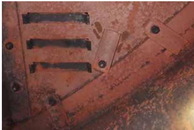
▲ Figure 17. A misoriented ring clip does not help hold the tray deck in place.
