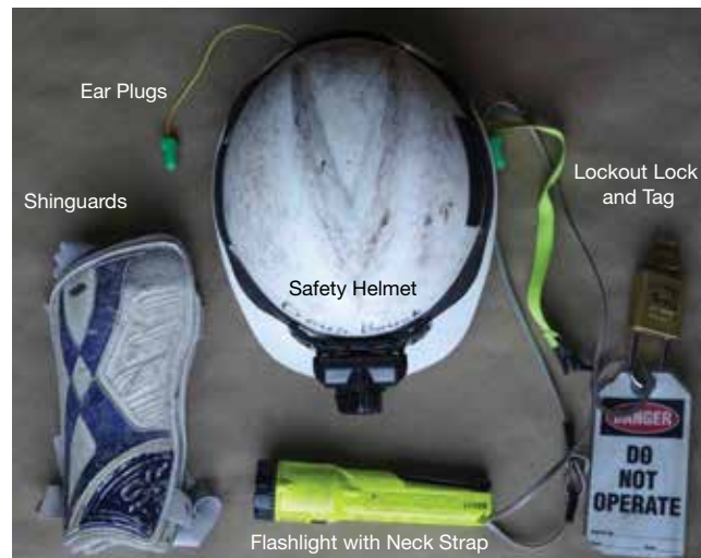
▲ Figure 5. I wear this safety equipment and bring my lockout lock and tag with me to all inspections.
