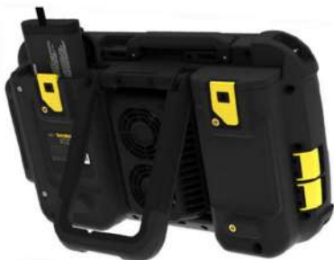
Figure 1 Rear of the instrument, showing the battery bays. The 2 yellow side lids each conceal the USB-C ports
