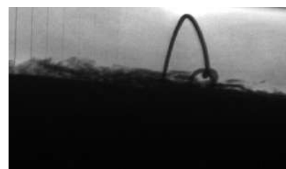
Figure B: Typical RTR image showing scale formation. The 'scaly' layer at the boundary between the pipe (black) and insulation (grey) depicts scale formation.
