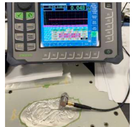
Figure 1 – Ultrasonic Thickness Mapping Inspection During Aircraft Heavy Maintenance
