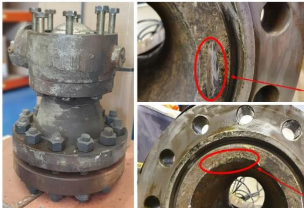
Figure 1 – Flange face defects
