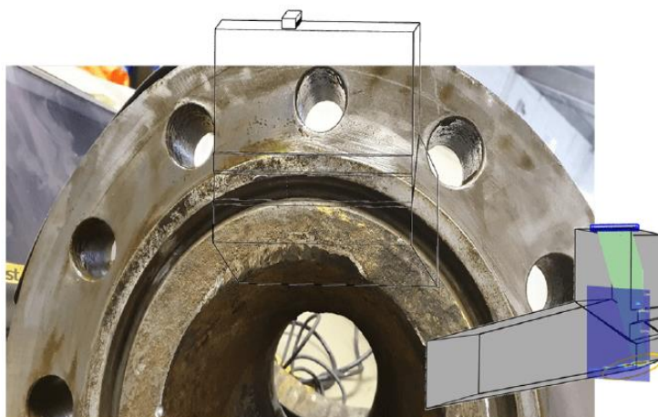
Figure 4 – Flange edge and its TFM scan location
