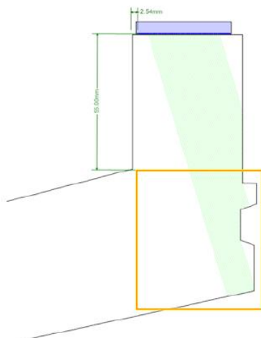
Figure 2 -Flange inspection scan plan
