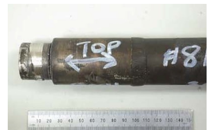
Figure-3, SRC of alloy 800HT inlet pigtail [8]
