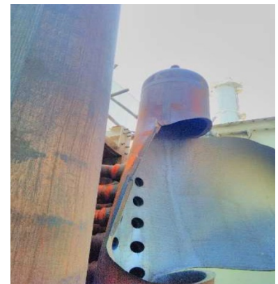
Figure 1 [Ruptured Superheater steam coil, SS316H by SRC [2]]- shows the rupture of a superheated steam coil outlet header, made from 48 mm thick SS316H, caused by stress relaxation cracking (SRC) at the longitudinal seam weld. The rupture resulted in extensive damage within the convection section of the steam reformer at a methanol plant. Additionally, large fragments of debris were projected up to 100 meters across the site, impacting surrounding areas [2]
