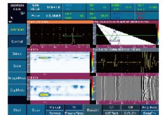
Simultaneous inspection of PAUT and TOFD can decrease undetected rate.
