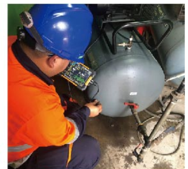
Ultrasonic thickness measurement
