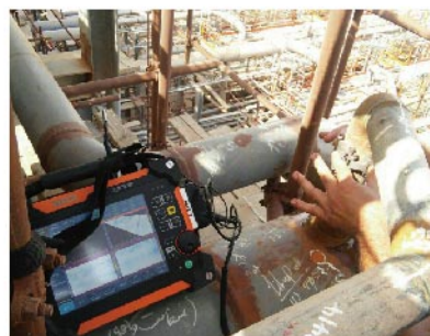
Tube weld inspection
