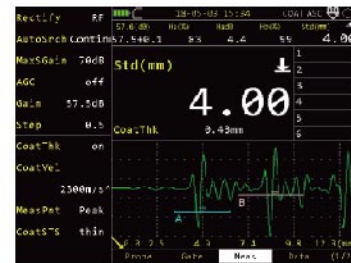
Coat and base material thickness can be displayed at the same time.
