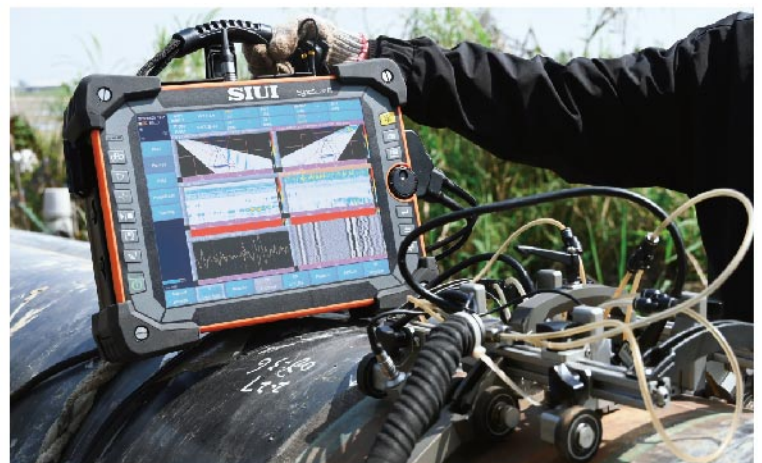
64-ch PA for 168mm thickness
